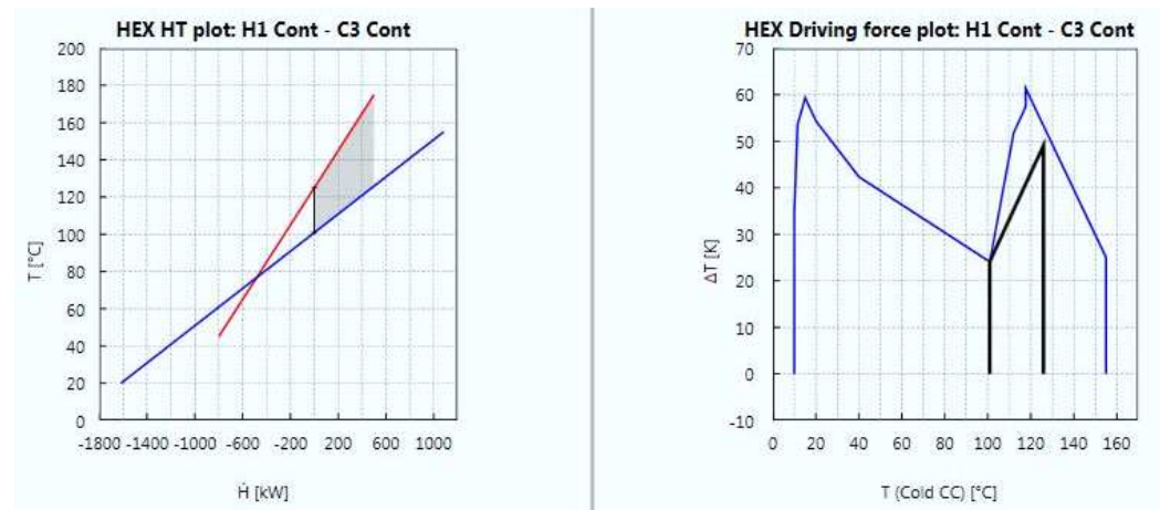
Fig. 12.8: Enthalpy versus Temperature Plot and Driving Force Plot
