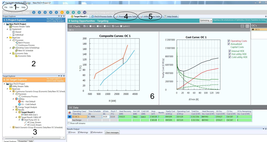
Fig. 3.2: PinCH Workbench and the major graphical components
