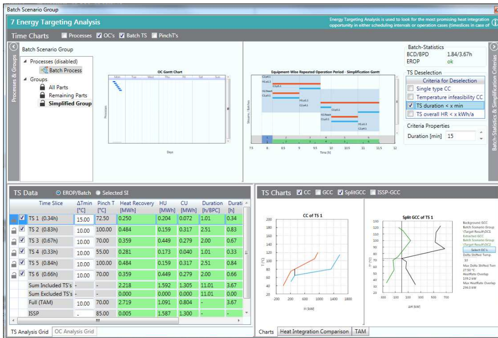
Fig. 9.2: ETA Single Product Batch visualizer showing the different analysis objects - OC Gantt Chart, Equipment Repeated Operation Period Gantt, TS Data grid and the TS Charts. Not displayed or hidden are the TAM charts, Heat Integration Comparison Charts, the split GCC Chart and the GCC based ISSP Chart.
