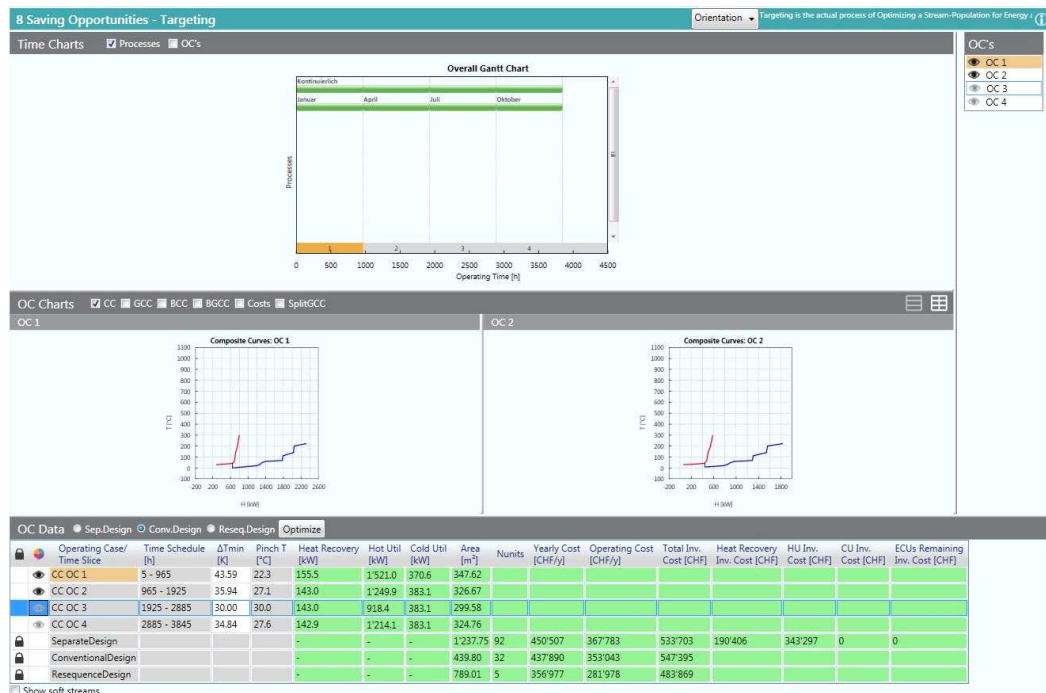
Fig. 8.10: MOC Combined Supertargeting Target Result showing the results for Conventional Design together with the summaries of the Separate Design and the Resequence Design types
